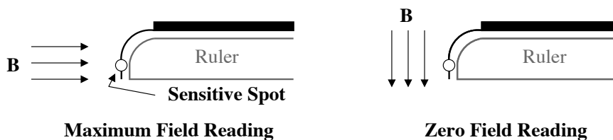
Figure 5.1: Measuring the magnetic field using the gaussmeter.
