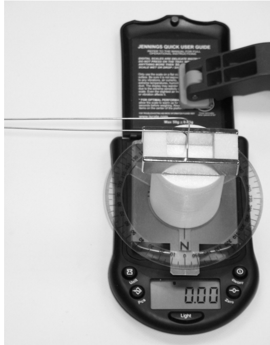
Figure 5.7: The magnetic field between the magnets points from one magnet to another, toward the "N" on the compass. Here the current and the magnetic field are parallel, so the net force is zero.
