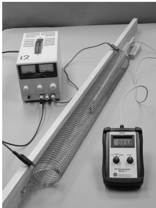
Figure 5.9: You can study the magnetic field of a solenoid using a Slinky and the gaussmeter.
