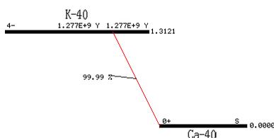
Figure 11.  $^{40}\text{K}$  decay scheme. (From P. M. Endt, *Nuclear Physics A521*, 1 (1990))
