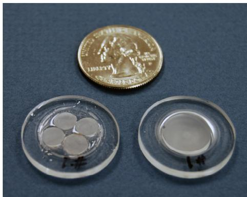
Figure 9. KCl crystals mounted on 1" diameter acrylic disks.
