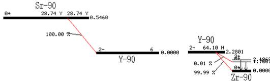
Figure 7.  $^{90}\text{Sr}$  -  $^{90}\text{Y}$  decay scheme. (From E. Browne, *Nuclear Data Sheet* **82**, 379 (1997))
