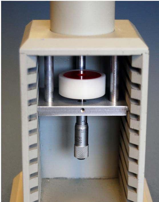
Figure 5. Equipment arrangement for  $\alpha$ -particle range measurements.
