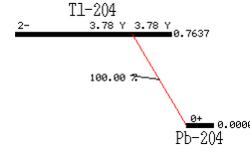
Figure 8.  $^{204}\text{Tl}$  decay scheme. (From M. R. Schmorak, *Nuclear Data Sheet* **72**, 409 (1994))
