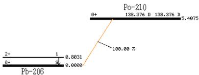
Figure 4.  $^{210}\text{Po}$  decay scheme. (From R. G. Helmer and M. A. Lee, *Nuclear Data Sheet* **61**, 93 (1990))
