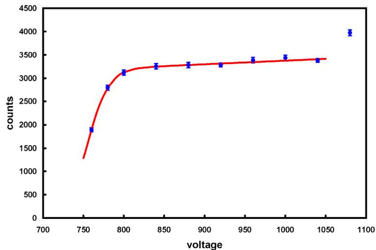
Figure 3. HV curve for a P2131 Geiger tube. The operating voltage was set at 920 v.
