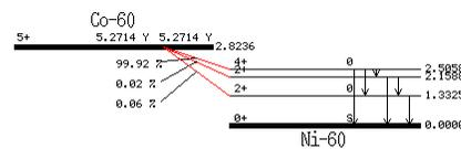
Figure 13.  $^{60}\text{Co}$  decay scheme. (From M. M. King, *Nuclear Data Sheet* **69**, 1 (1993))
