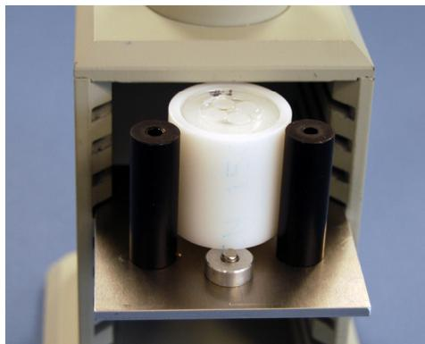
Figure 10. KCl sample on Delrin support ready to be inserted under Geiger counter.
