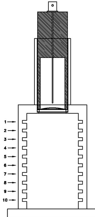
Figure 1. The Geiger counter and support assembly. The numbers 1 – 10 label slots for inserting sources and absorbers.
