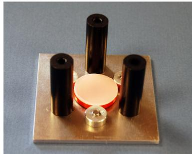
Figure 14. Gamma-ray source with 1/16"  $\text{CH}_2$  absorber.
