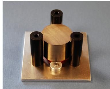
Figure 15. Gamma-ray source with stacked W absorbers.
