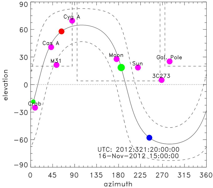
Figure 4. The graphic output of the IDL program, *radio\_coords*. The green dots indicate the Galactic center (large) and the Galactic anti-center (small). The red and blue dots point to galactic longitudes of  $90^\circ$  and  $270^\circ$  respectively. The sky coverage accessible to the antenna mount lies above the straight dashed lines. The difference between local time and GMT (UTC) is either 4 hours (in the summer) or 5 hours (in the winter).
