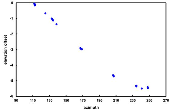
Figure 5b. Elevation axis errors determined from solar observations.
