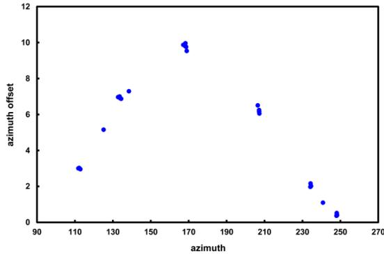
Figure 5a. Azimuth axis errors determined from solar observations.
