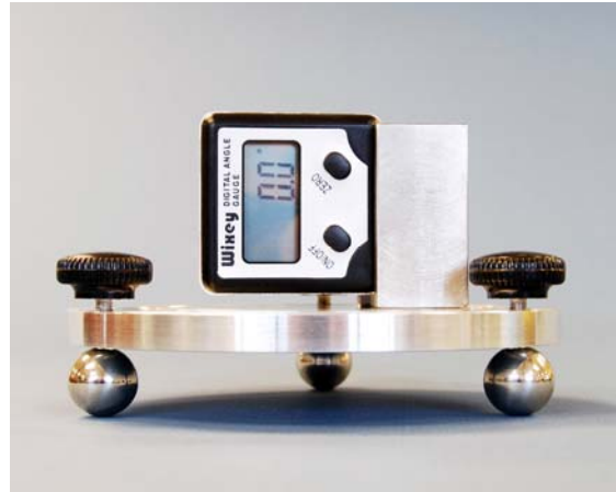
Figure 10. Leveling table with steel block to set the Wixey digital angle gauge reference direction to vertical.
