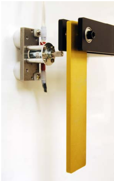
Figure 12. Pendulum period test configuration (a).
