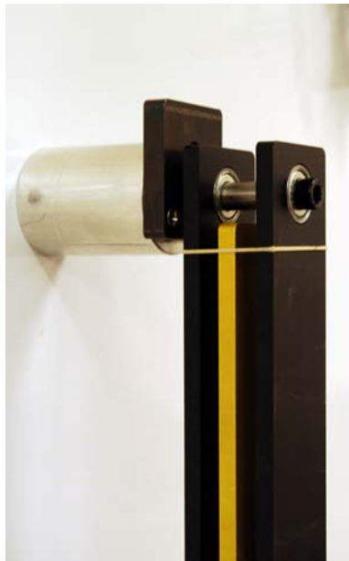
Figure 13. Pendulum period test configuration (b).
