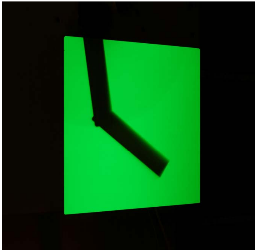
Figure 5. The shadow image of the double pendulum caught by the electronic flash gun.
