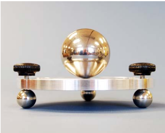
Figure 9. Leveling table with 2" diameter steel ball. Adjust screws until ball position is neutral.
