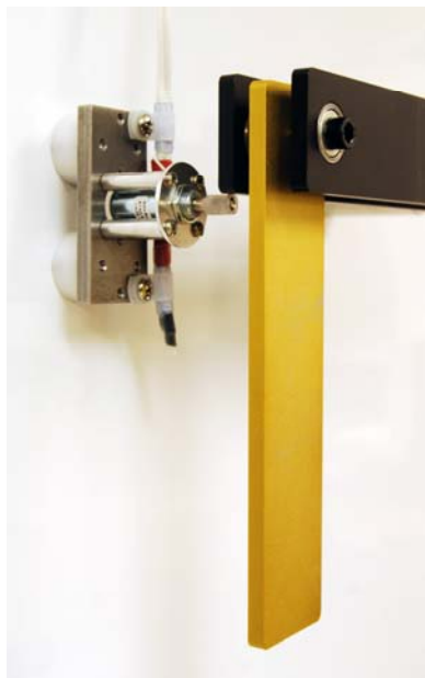
Figure 12. Pendulum period test configuration (a).
