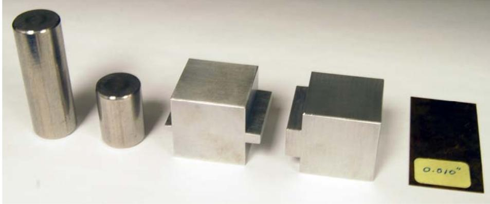
Figure 3. Spacer blocks for source displacement measurement and collimator width alignment. From left to right: 1.80" steel spacer rod, 0.90" steel spacer rod, 0.75 and 2.50 mm collimator alignment tool, 10.0 mm collimator alignment tool, 0.010" collimator alignment tool.
