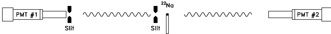
Figure 3. Arrangement of collimation slits to determine the \beta^+ spatial distribution within the ^{22}\text{Na} source holder.
